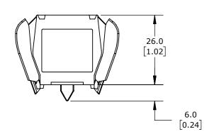
22mm, (1) N.C. CONTACT(s). PACKAGE OF 2. FOR USE WITH ECX4029-2 MOUNTING FLANGE.
