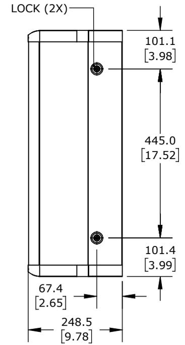
TEKNOKOL ECO SERIES HMI ENCLOSURE, 20 X 24 X 9IN (HXWXD), SUSPENSION MOUNT, ALUMINUM, NATURAL FINISH, SCREW COVER.
