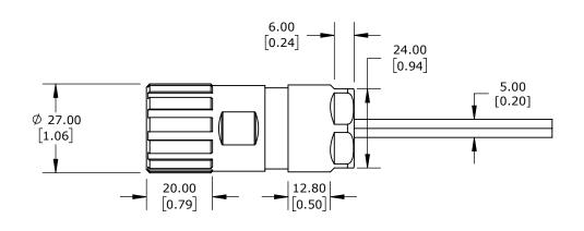
LIKA ELECTRONIC ENCODER CABLE, M23 AXIAL FEMALE TO PIGTAIL, SHIELDED, 16.4FT/5M CABLE LENGTH, FOR USE WITH LIKA ELECTRONIC A80 SERIES ENCODERS
