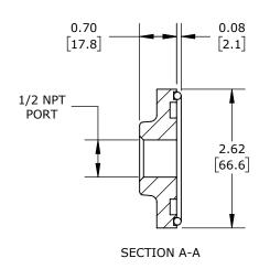
1/2IN FEMALE NPT. FOR USE WITH CITO STACKFLOW VALVES BODY INLET. BK-9100 BOLT KIT INCLUDED.
