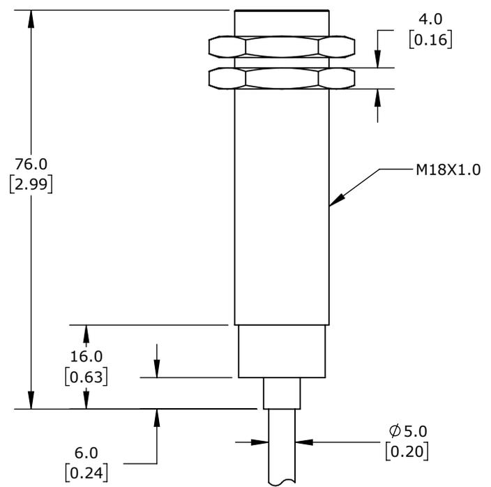
CONTRINEX INDUCTIVE PROXIMITY SENSOR, TUBULAR, 18MM DIAMETER X 76MM BODY, 304 STAINLESS STEEL HOUSING, PNP, N.O., 5MM SENSING DISTANCE, FLUSH, 400 HZ SWITCHING FREQUENCY, IP67, PIGTAIL.
