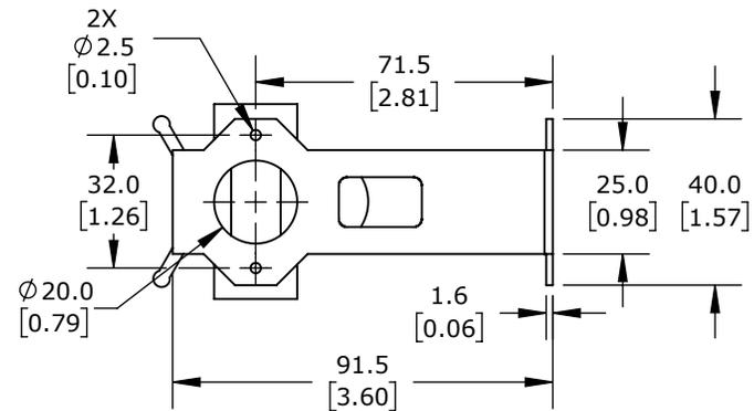
PROSENSE PANEL MOUNT BRACKET, FOR USE WITH DPM2 AND DPM3 SERIES 1/8 DIN
