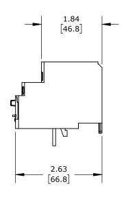
7-10A ADJUSTABLE, BI-METALLIC, DIRECT MOUNT POWER CONNECTION(s). FOR USE WITH SCHNEIDER ELECTRIC DPE09 TO DPE38 CONTACTORS.
