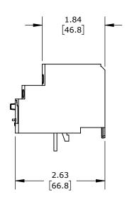
0.40-0.63A ADJUSTABLE, BI-METALLIC, DIRECT MOUNT POWER CONNECTION(s). FOR USE WITH SCHNEIDER ELECTRIC DPE09 TO DPE38 CONTACTORS.
