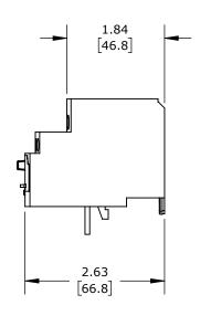
0.25-0.40A ADJUSTABLE, BI-METALLIC, DIRECT MOUNT POWER CONNECTION(s). FOR USE WITH SCHNEIDER ELECTRIC DPE09 TO DPE38 CONTACTORS.
