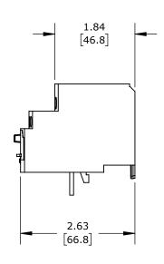
0.16-0.25A ADJUSTABLE, BI-METALLIC, DIRECT MOUNT POWER CONNECTION(s). FOR USE WITH SCHNEIDER ELECTRIC DPE09 TO DPE38 CONTACTORS.
