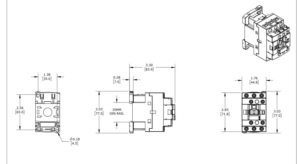
25A, (3) N.O. POWER POLES, (1) N.O. AUXILIARY CONTACTS, 120 VAC (50/60Hz) COIL VOLTAGE.
