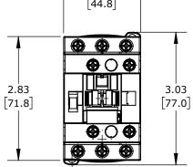
18A, (3) N.O. POWER POLES, (1) N.O. AUXILIARY CONTACTS, 24 VDC COIL VOLTAGE.
