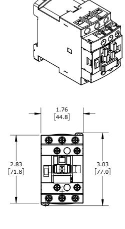
9A, (3) N.O. POWER POLES, (1) N.O. AUXILIARY CONTACTS, 24 VDC COIL VOLTAGE.
