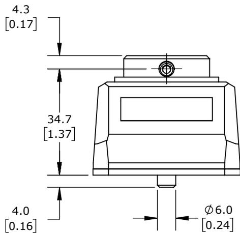
ELESA POSITION INDICATOR, 5-DIGIT MECHANICAL, INCLINED LOWER, 000.50 COUNTS PER REVOLUTION, COUNTER CLOCKWISE, 20MM MOUNTING HOLE SIZE, IP65.
