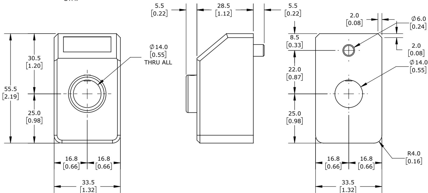
ELESA POSITION INDICATOR, 8MM 5-DIGIT LCD, PROGRAMMABLE, 14MM MOUNTING HOLE SIZE, IP67.
