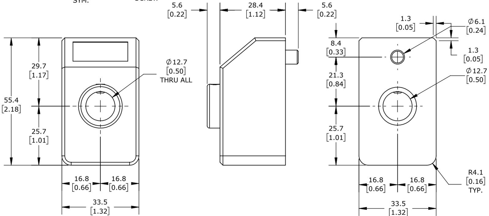
ELESA POSITION INDICATOR, 8MM 5-DIGIT LCD, PROGRAMMABLE, 1/2IN MOUNTING HOLE SIZE, IP65.
