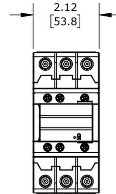
50A, (3) N.O. POWER POLES, (3) N.O./ (3) N.C. SAFETY AUXILIARY CONTACTS, 24 VAC (50/60Hz) COIL VOLTAGE.
