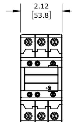
50A, (3) N.O. POWER POLES, (3) N.O./ (3) N.C. SAFETY AUXILIARY CONTACTS, 24 VDC COIL VOLTAGE.
