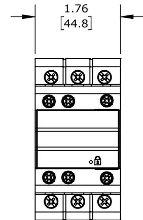
32A, (3) N.O. POWER POLES, (3) N.O./ (3) N.C. SAFETY AUXILIARY CONTACTS, 24 VDC COIL VOLTAGE.
