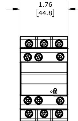
18A, (3) N.O. POWER POLES, (3) N.O./ (3) N.C. SAFETY AUXILIARY CONTACTS, 24 VDC COIL VOLTAGE.
