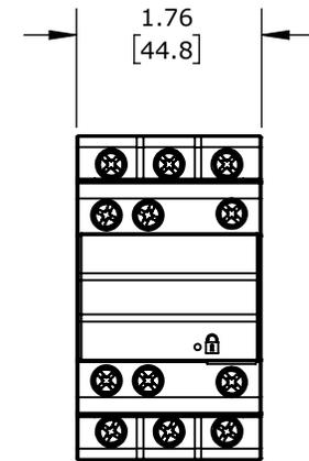
12A, (3) N.O. POWER POLES, (3) N.O./ (3) N.C. SAFETY AUXILIARY CONTACTS, 120 VAC (50/60Hz) COIL VOLTAGE.
