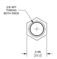
PNEUMATIC, COOLANT, OIL OR WATER THREADED FITTING, FEMALE, CHECK VALVE, BRASS BODY, BRASS THREADS, (2) 3/8IN FEMALE NPT.
