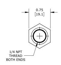
PNEUMATIC, COOLANT, OIL OR WATER THREADED FITTING, FEMALE, CHECK VALVE, BRASS BODY, BRASS THREADS, (2) 1/4IN FEMALE NPT.
