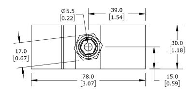
LAUMAS TENSION AND COMPRESSION LOAD CELL, 1102 LB/500 KG, +/- 0.02% OF FULL SCALE ACCURACY, VOLTAGE SIGNAL RANGE(s) OF 2 MV/V, 3-15 VDC, STAINLESS STEEL, IP68, 32.8FT/10M INTEGRAL 6-WIRE SHIELDED CABLE
