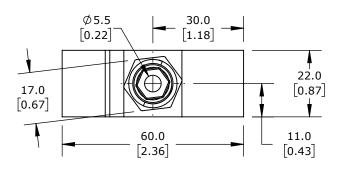
LAUMAS TENSION AND COMPRESSION LOAD CELL, 660 LB/300 KG, +/- 0.02% OF FULL SCALE ACCURACY, VOLTAGE SIGNAL RANGE(s) OF 2 MV/V, 3-15 VDC, STAINLESS STEEL, IP68, 32.8FT/10M INTEGRAL 6-WIRE SHIELDED CABLE
