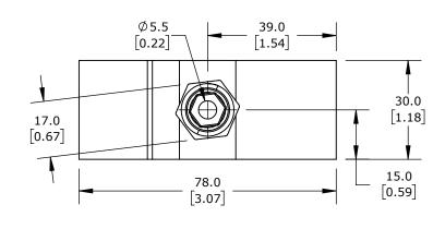
LAUMAS TENSION AND COMPRESSION LOAD CELL, 5510 LB/2500 KG, +/- 0.02% OF FULL SCALE ACCURACY, VOLTAGE SIGNAL RANGE(s) OF 2 MV/V, 3-15 VDC, STAINLESS STEEL, IP68, 32.8FT/10M INTEGRAL 6-WIRE SHIELDED CABLE
