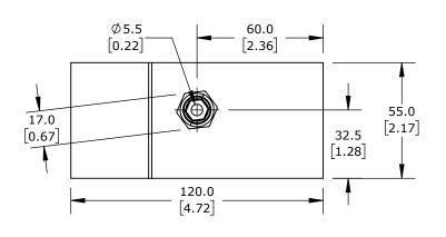
LAUMAS TENSION AND COMPRESSION LOAD CELL, 27550 LB/12500 KG, +/- 0.02% OF FULL SCALE ACCURACY, VOLTAGE SIGNAL RANGE(s) OF 2 MV/V, 3-15 VDC, STAINLESS STEEL, IP68, 32.8FT/10M INTEGRAL 6-WIRE SHIELDED CABLE
