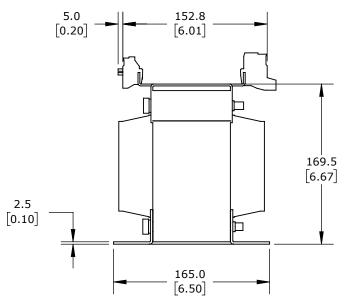
OPEN CORE, 2 KVA, 1-PHASE, 240/480 VAC PRIMARY, 120 VAC SECONDARY, 50/60 Hz, PANEL MOUNT.
