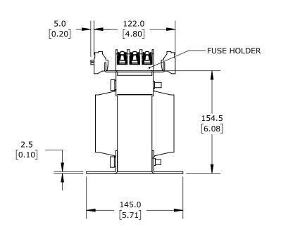
OPEN CORE, 1 KVA, 1-PHASE, 240/480 VAC PRIMARY, 120 VAC SECONDARY, 50/60 Hz, FUSED, PANEL MOUNT.
