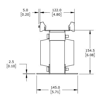
OPEN CORE, 1 KVA, 1-PHASE, 240/480 VAC PRIMARY, 120 VAC SECONDARY, 50/60 Hz, PANEL MOUNT.
