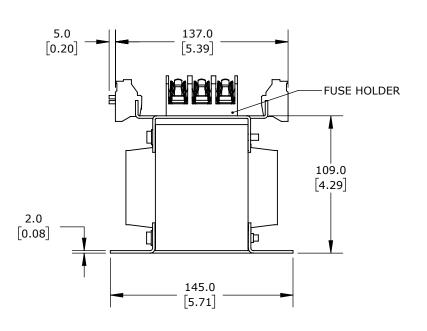
OPEN CORE, 500 VA, 1-PHASE, 240/480 VAC PRIMARY, 120 VAC SECONDARY, 50/60 Hz, FUSED, PANEL MOUNT.
