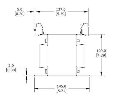
OPEN CORE, 500 VA, 1-PHASE, 240/480 VAC PRIMARY, 120 VAC SECONDARY, 50/60 Hz, PANEL MOUNT.
