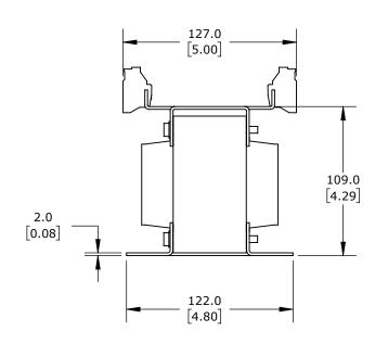
OPEN CORE, 350 VA, 1-PHASE, 600 VAC PRIMARY, 24 VAC SECONDARY, 50/60 Hz, PANEL MOUNT.
