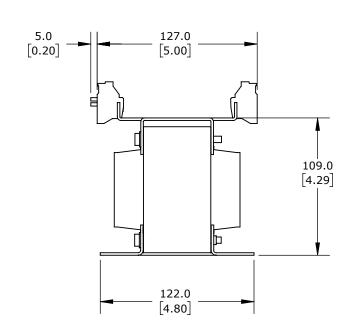
OPEN CORE, 350 VA, 1-PHASE, 240/480 VAC PRIMARY, 24 VAC SECONDARY, 50/60 Hz, PANEL MOUNT.
