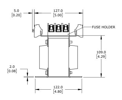
OPEN CORE, 350 VA, 1-PHASE, 240/480 VAC PRIMARY, 120 VAC SECONDARY, 50/60 Hz, FUSED, PANEL MOUNT.
