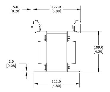
OPEN CORE, 350 VA, 1-PHASE, 240/480 VAC PRIMARY, 120 VAC SECONDARY, 50/60 Hz, PANEL MOUNT.
