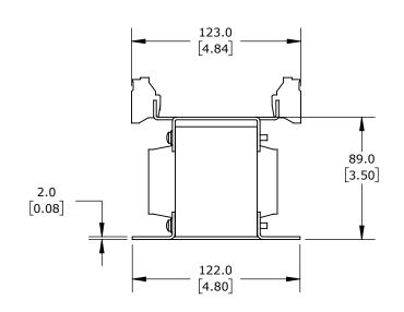
OPEN CORE, 250 VA, 1-PHASE, 600 VAC PRIMARY, 24 VAC SECONDARY, 50/60 Hz, PANEL MOUNT.
