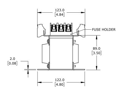
OPEN CORE, 250 VA, 1-PHASE, 600 VAC PRIMARY, 120 VAC SECONDARY, 50/60 Hz, FUSED, PANEL MOUNT.
