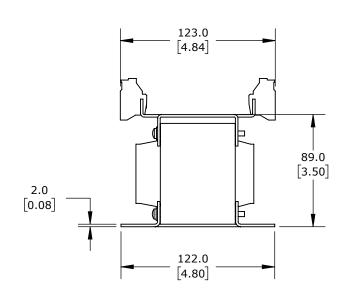
OPEN CORE, 250 VA, 1-PHASE, 600 VAC PRIMARY, 120 VAC SECONDARY, 50/60 Hz, PANEL MOUNT.
