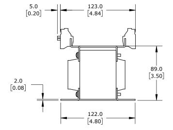
OPEN CORE, 250 VA, 1-PHASE, 240/480 VAC PRIMARY, 24 VAC SECONDARY, 50/60 Hz, PANEL MOUNT.
