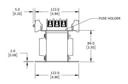
OPEN CORE, 250 VA, 1-PHASE, 240/480 VAC PRIMARY, 120 VAC SECONDARY, 50/60 Hz, FUSED, PANEL MOUNT.
