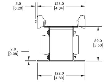
OPEN CORE, 250 VA, 1-PHASE, 240/480 VAC PRIMARY, 120 VAC SECONDARY, 50/60 Hz, PANEL MOUNT.
