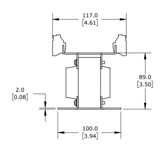
OPEN CORE, 150 VA, 1-PHASE, 600 VAC PRIMARY, 120 VAC SECONDARY, 50/60 Hz, PANEL MOUNT.
