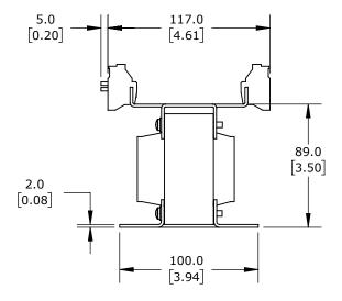
OPEN CORE, 150 VA, 1-PHASE, 240/480 VAC PRIMARY, 24 VAC SECONDARY, 50/60 Hz, PANEL MOUNT.
