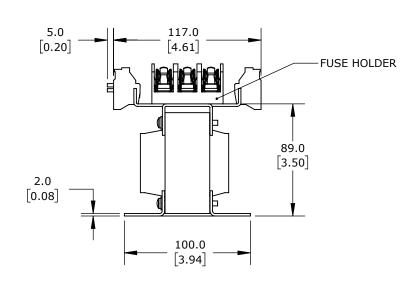
OPEN CORE, 150 VA, 1-PHASE, 240/480 VAC PRIMARY, 120 VAC SECONDARY, 50/60 Hz, FUSED, PANEL MOUNT.
