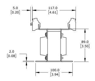
OPEN CORE, 150 VA, 1-PHASE, 240/480 VAC PRIMARY, 120 VAC SECONDARY, 50/60 Hz, PANEL MOUNT.
