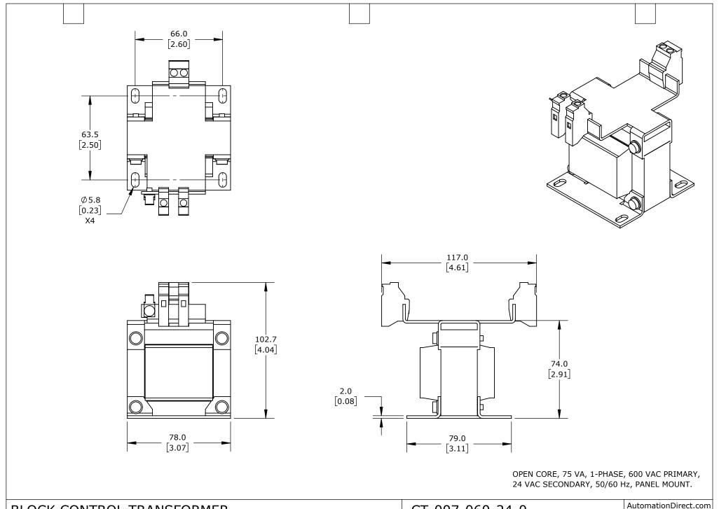
**BLOCK CONTROL TRANSFORMER** CT-007-060-24-0 1-800-633-0405 UNLESS OTHERWISE 3rd PART DIMENSIONS MAY DIFFER SLIGHTLY METRIC UNITS USED LATEST VERSION NOT TO mm SHEET 1 OF 1 ANGLE SPECIFIED UNITS ARE: [inch] 10/31/2024 SCALE FOR PART DESIGN DUE TO MANUFACTURER'S VARIANCES
