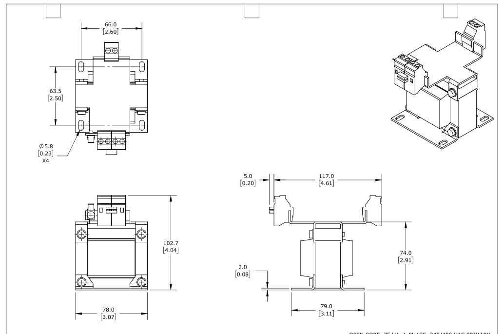
OPEN CORE, 75 VA, 1-PHASE, 240/480 VAC PRIMARY, 24 VAC SECONDARY, 50/60 Hz, PANEL MOUNT.
