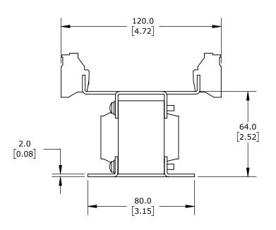
OPEN CORE, 50 VA, 1-PHASE, 600 VAC PRIMARY, 24 VAC SECONDARY, 50/60 Hz, PANEL MOUNT.
