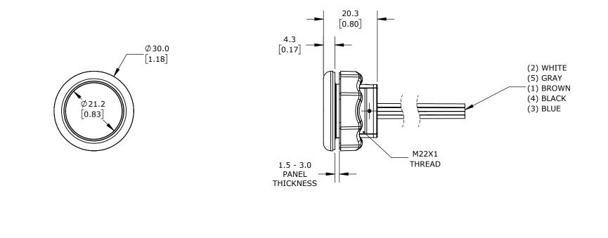
STANDARD CAPACITIVE PUSHBUTTON SENSOR SWITCH, IP69K, 22mm, STATIC, POLYCARBONATE BEZEL, SEMI-AUTOMATIC LED CONTROL, OPERATOR: WHITE, 30mm.
